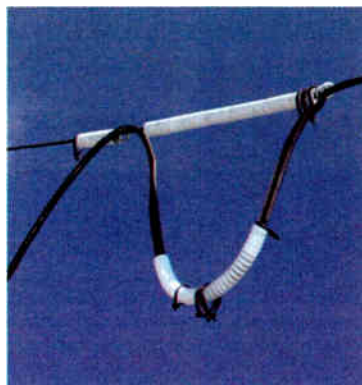
Ferrites block the RF on the line.
