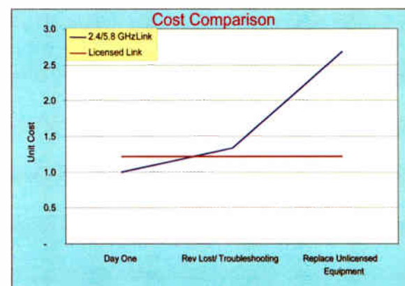
Unlicensed solutions have low initial cost, but typically a higher long-term cost when operations and interference are accounted for.
