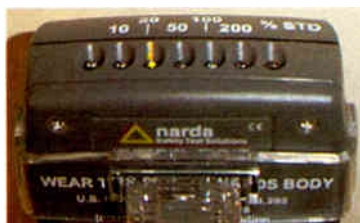
Checking RFR levels at the transmitter building wall near to the tower.
