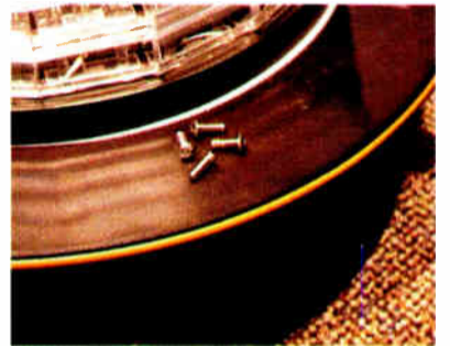
Six of these tiny screws are all that holds the beacon to the tower.
