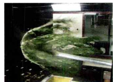
Two 8-foot eucalyptus branches subjected to 150 mph wind in a wind tunnel. Photo: Chameleon Engineering
