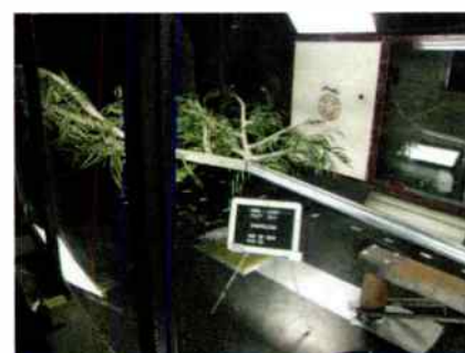
Two 8-foot eucalyptus branches in a wind tunnel prior to testing. Photo: Chameleon Engineering
