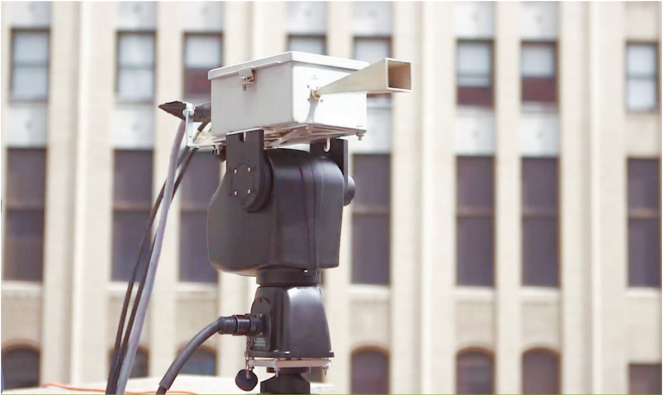
To directoinalize the signal the way a large array antenna could, the signal appratus was fitted with a horn antenna. Photo courtesy of IEEE Access
