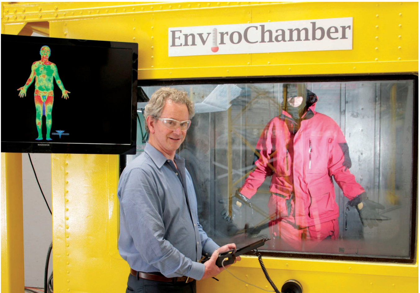
Art Seely, founder and CEO of Safety One Training International, is operating the company's envirochamber where tower-climbing students can test various types of insulating and outer protective layer garments at temperatures of -10° F and wind speeds up to 50 miles per hour.
