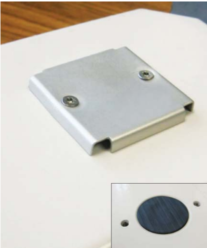
Photo 1. Adhesive vent position on sample equipment.
