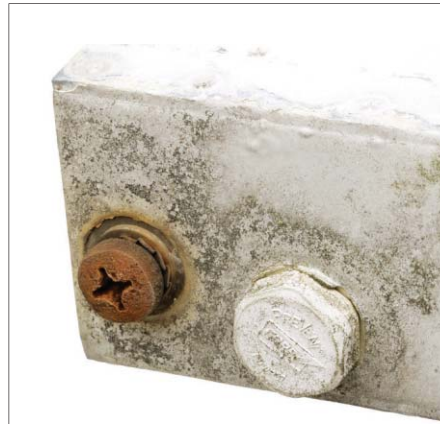
Photo 2. Screw-in vent position on sample equipment.
