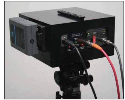
The GigaLink HD wireless radio links are available as single or dual channel. They are the first unlicensed wireless system that transmits uncompressed HD/SDI video at 1.485 GB/s. The unit shown above is a receiver.
