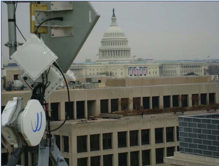
An 80-GHz Gigabit Ethernet medium-range wireless bridge from BridgeWave Communications extends a backhaul connection for as much as three miles.
