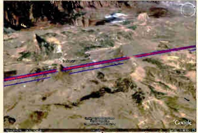
Figure 4. These two views of proposed radio signal paths indicate that the terrain is severely blocking the reception on this path. Software allows the designer to know in advance if these problems will be present and to make design adjustments to eliminate or minimize these types of problems.
