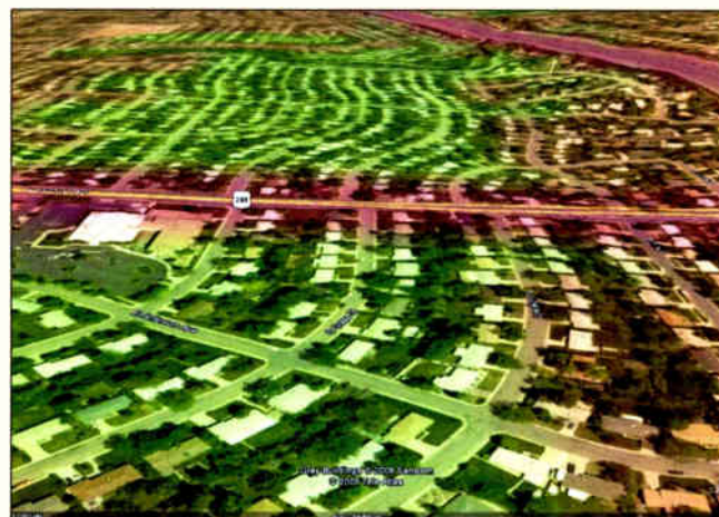
Figure 3. These graphics represent a close-up view of the received signal levels on both sides of Hampden Ave. in the Denver, Colo., area. Note the lower elevations off to the right (red) where the signal level is reduced below what is present in the residential areas that are higher in elevation (green).
