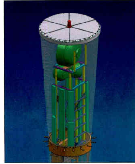
Positioning a radio base station at an elevation inside the tube reduces low feeder loss, which in turn allows improved network coverage and capacity.
