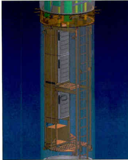
Equipment designed for use indoors can be used inside the tube. A radome protects antennas. The concrete shell adds protection from vandalism and lightning.
