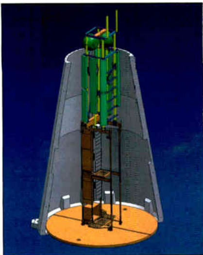
Radio base stations are initially installed at the bell-shaped base of the tower and then raised to the top by an elevator.
