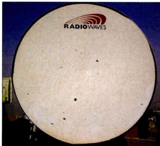
The Radio Waves microwave dish shown in two views at the left was struck by debris from a 107 mm rocket that impacted the corner of the rooftop shown at the right. The antenna was installed at a forward operating base in Iraq. The antenna at the right is of unknown manufacture. Photo: 'Steve'in Iraq; www.microwaves101.com.
