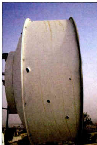
The Radio Waves microwave dish shown in two views at the left was struck by debris from a 107 mm rocket that impacted the corner of the rooftop shown at the right. The antenna was installed at a forward operating base in Iraq. The antenna at the right is of unknown manufacture. Photo: 'Steve'in Iraq; www.microwaves101.com.
