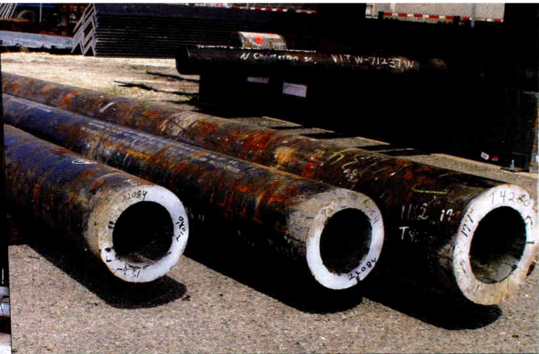
Concealment poles such as flagpoles, trees and custom structures, begin their fabrication process at Stealth Concealment Solutions as raw steel tubes. The factory has tools for steel punching and shearing, automated steel cutting, and welding.
