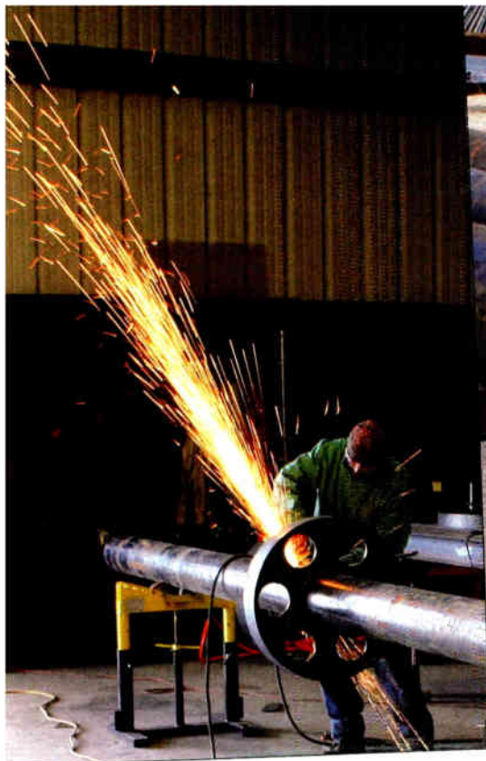
Concealment poles such as flagpoles, trees and custom structures, begin their fabrication process at Stealth Concealment Solutions as raw steel tubes. The factory has tools for steel punching and shearing, automated steel cutting, and welding.
