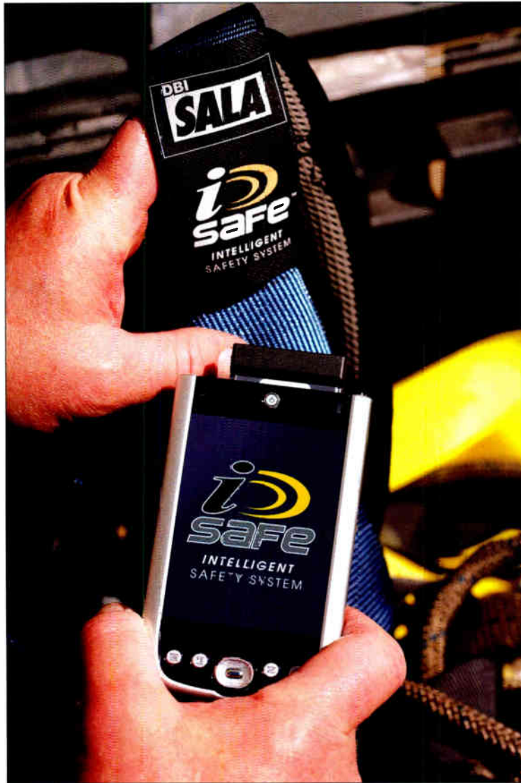
Tags are read by a portable site PDA that scans the piece of equipment and accounts for it by a unique number. The readers make for easy entry to log inspections, equipment assignments by worker or location, and more.
