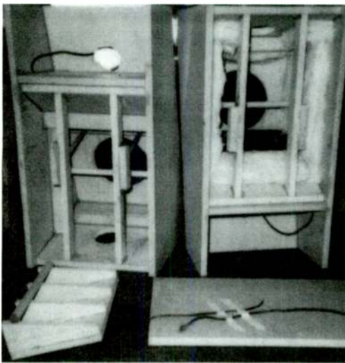
PHOTO 8: Woofer box back braces and damping material.
