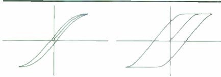
FIGURE 2: Hysteresis loops for soft iron (left) and hard iron (right).
