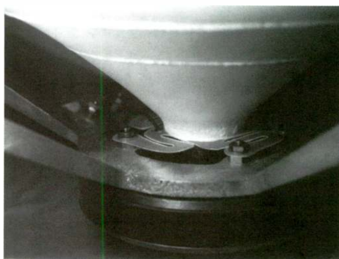
PHOTO 4: "S"-shaped spider construction.
