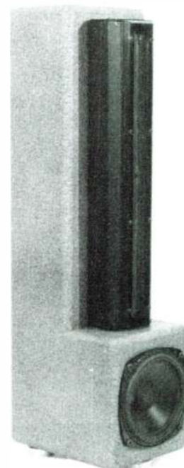
PHOTO 2: Module 15, with 15" ribbon crossed to a 4Ω Peerless 5" at approximately 1.2kHz. Ribbon impedance is 6Ω; sensitivity is 87dB.
