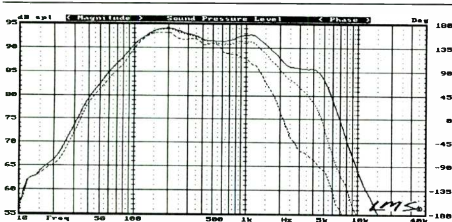
FIGURE 3: Off-axis response. Even a 5" driver is down over 12dB at 2k at 90° and 18dB at 3k. That is why a low crossover is so critical to consistent off-axis response and hence to the integrity of the soundstage. The larger the bass driver, the greater the midrange suckout off-axis. I used a single inductor and smoothed the curves heavily to get rid of the trash and concentrate on the issue.
