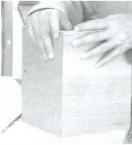
PHOTO 6: Note the smooth, clean joint along the outside edge of this corner spline joint.
