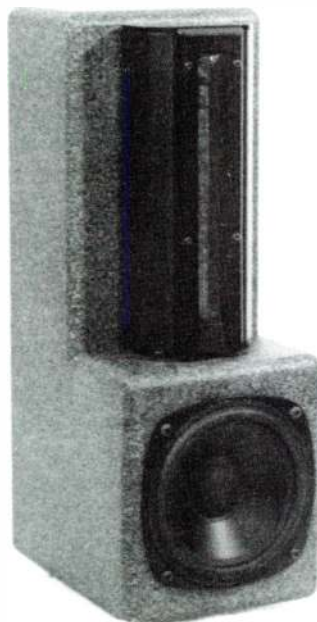
PHOTO 1: Module 8, with 8" ribbon crossed over to an 8Ω 5" Peerless mid-bass at approximately 1.3kHz. Ribbon impedance is 11Ω; sensitivity is 85dB.
