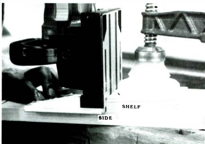
PHOTO 12: Making the vertical cut into the side piece: an interior butt joint.
