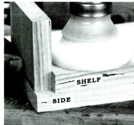
PHOTO 7: Aligning and clamping the pieces together: corner joint.
