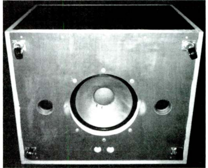
PHOTO 2: Bottom view of enclosure (mounted on casters) showing the placement of two ducts in relation to driver.
