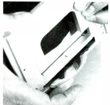
PHOTO 2: Adjusting the depth of cut on the biscuit joiner.
