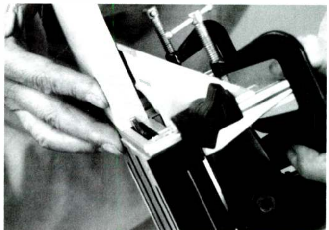
PHOTO 4: Adjusting to center the slot cut. Notice the clamps holding the fence firmly in place.
