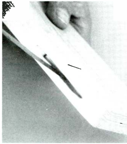
PHOTO 6: Spreading the glue in a slot with a palette knife.
