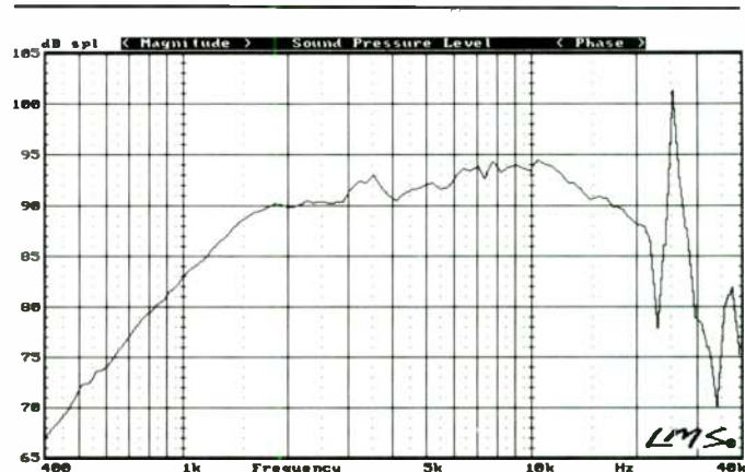
FIGURE 11: Tweeter on-axis frequency response.
