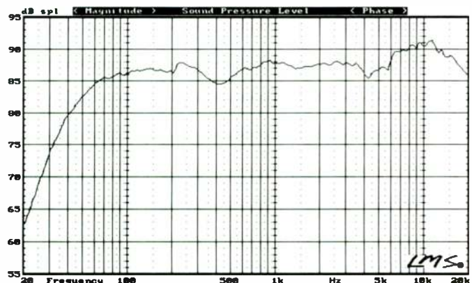
FIGURE 14: Full-range on-axis system frequency response (does not include rear port radiation).
