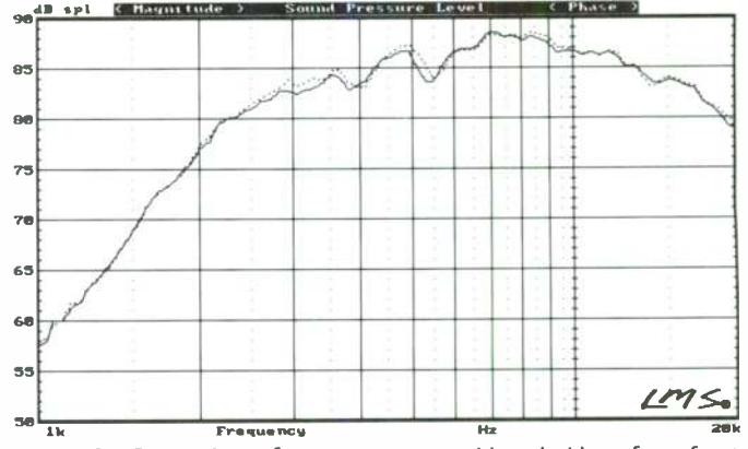
FIGURE 34: Comparison of tweeter response with and without foam front baffle damping material at 15° off axis (solid = with foam, dash = without foam).
