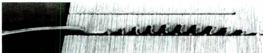
PHOTO 3: Fine-cutting plywood saw blade set with the gullet of the teeth at the surface of the plywood.
