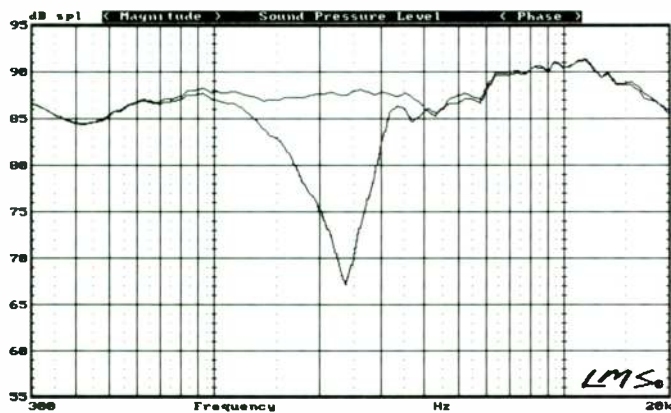
FIGURE 20: Frequency response comparison, in phase and tweeter electrically out of phase.
