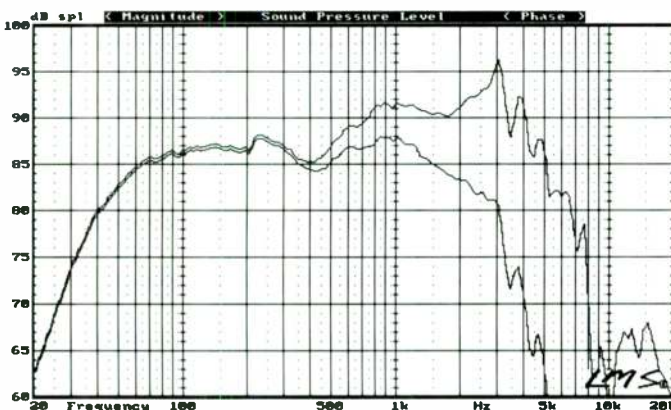
FIGURE 8: Woofer response with and without low-pass network.
