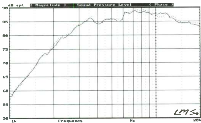
FIGURE 33: Comparison of tweeter response with and without foam front baffle damping material at 0° (solid = with, dash = without).
