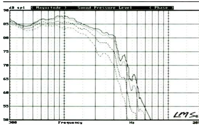
FIGURE 10: Woofer frequency response with low-pass network (solid = 0°, dot = 15°, dash = 30°, dash/dot = 45°).
