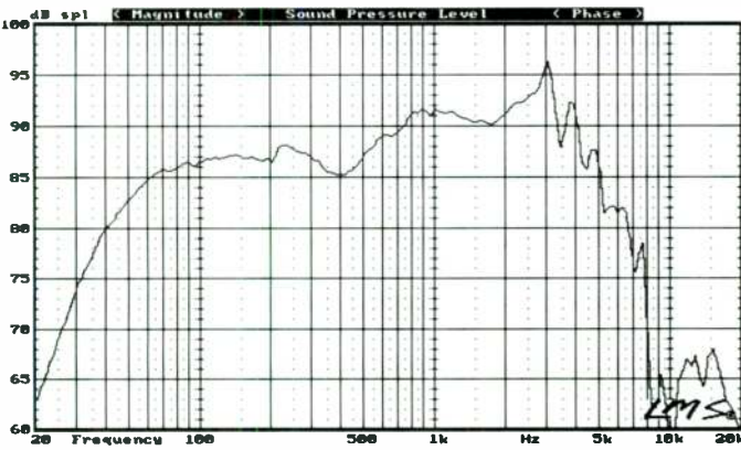
FIGURE 4: Woofer full-range on-axis anechoic frequency response (does not include rear port radiation).
