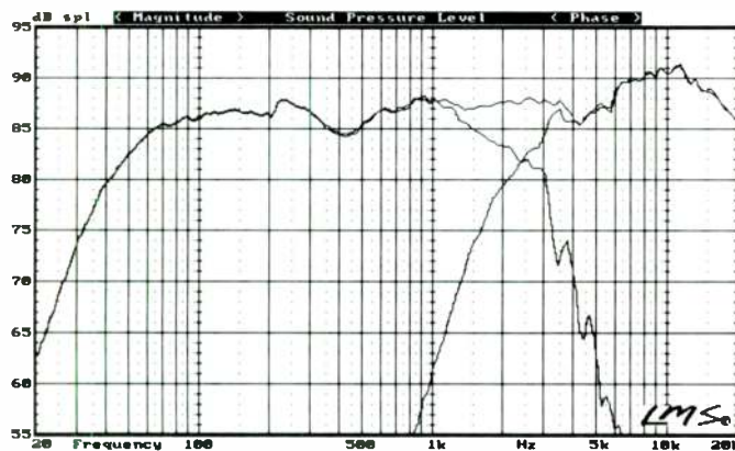
FIGURE 19: Woofer, tweeter, and system frequency-response graph.
