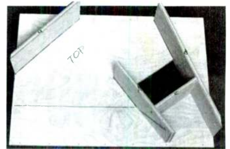
PHOTO 2: Throat partitions mounted to the top.
