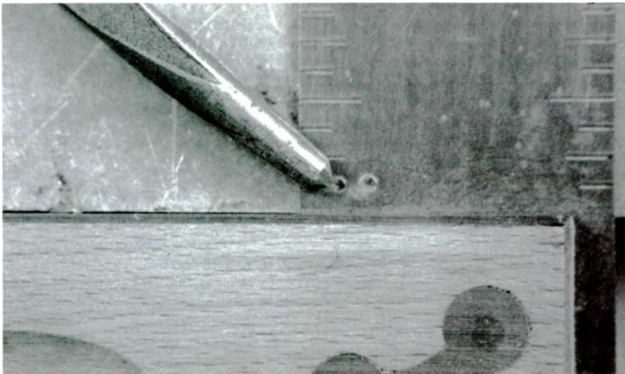
PHOTO 3: Peening the blade of the try square to obtain alignment.
