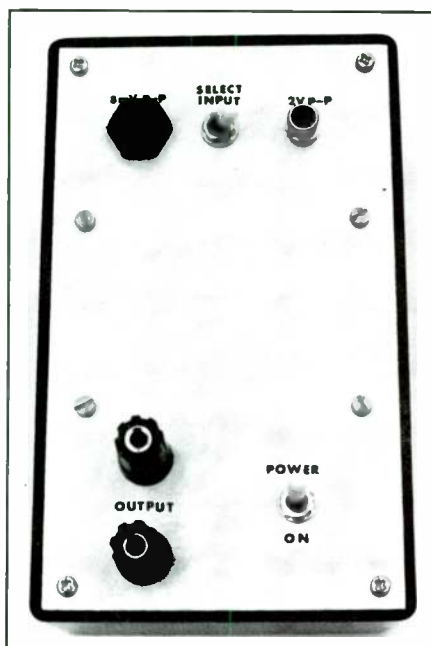
PHOTO 4: Panel of the level monitor.
