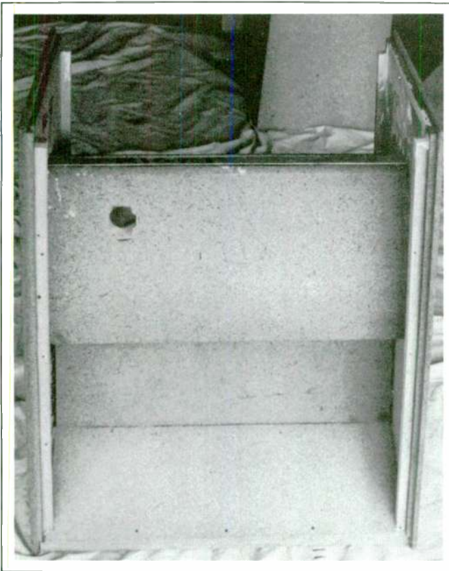
PHOTO 7: Front of center "snail" section, fully assembled. Note hole in panel for midrange horn.
