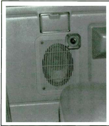
PHOTO 2: Finished rear tweeter installation.
