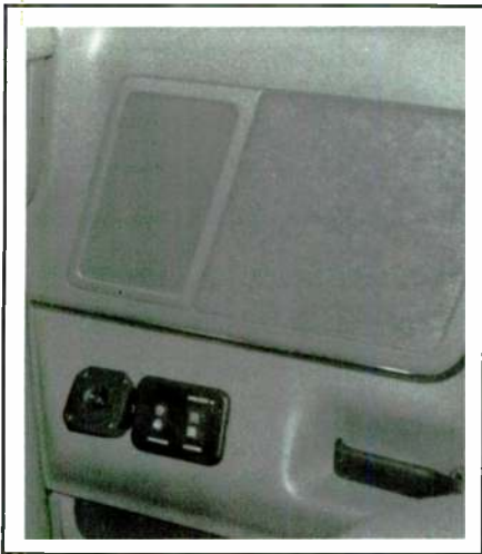
PHOTO 1: Finished front tweeter installation.
