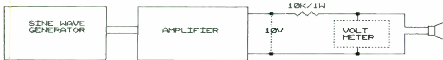
FIGURE 3: Setup for measuring speaker impedance. Adjust the amplifier volume control for an output of 10V across the 1kΩ resistor when the speaker terminals are shorted out. Then hook up the speaker and measure the voltage across its terminals. A 10Ω impedance should give 100mV, a 20Ω impedance 200mV, and so on.
