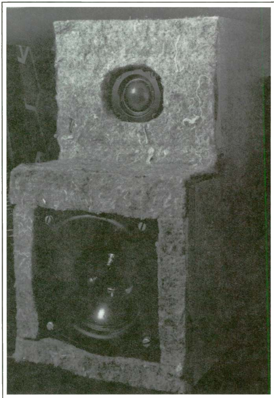
PHOTO 1: Satellite enclosures, reworked to set back the D-28AF.
