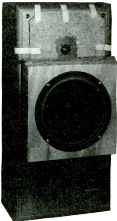
PHOTO A: The modified speaker without its grille cloth.
