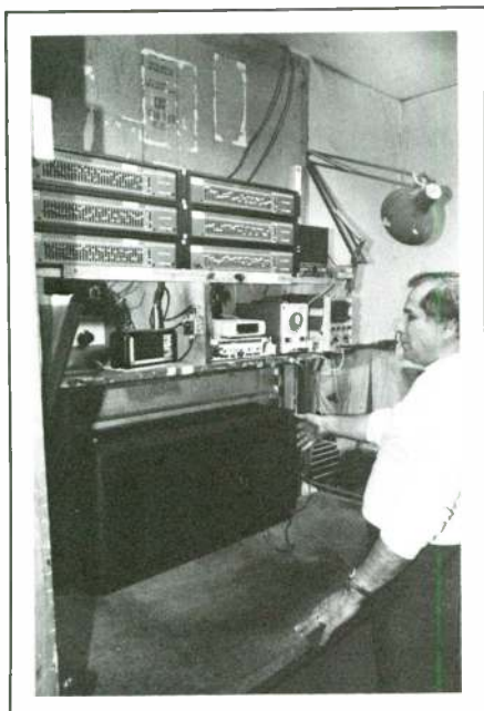
FIGURE 17: Every completed speaker is checked in a chamber for frequency response.
