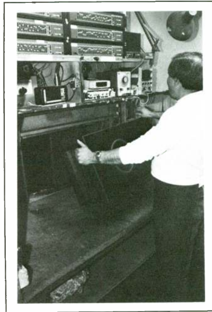
FIGURE 18: The operator then turns the speaker around and checks the response sweep with his ear for rattles, buzzes, and any other distortion.
