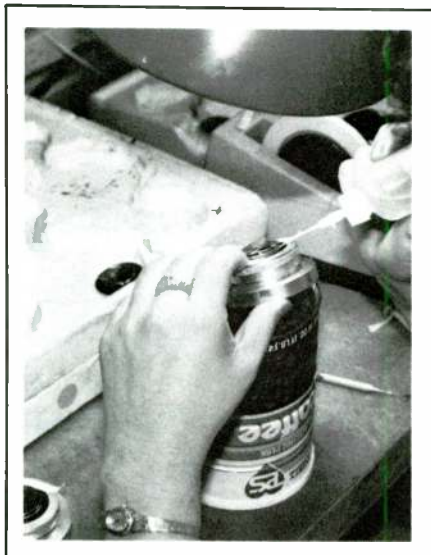
FIGURE 11: The tweeter production begins with attaching the voice coil to the diaphragm with a specialized adhesive.
