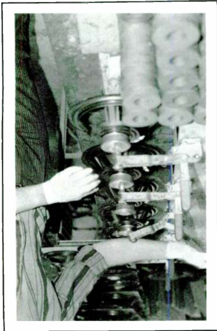
FIGURE 3: Woofer production begins by attaching the magnet-pole piece assembly to the basket with a quick-setting adhesive.
