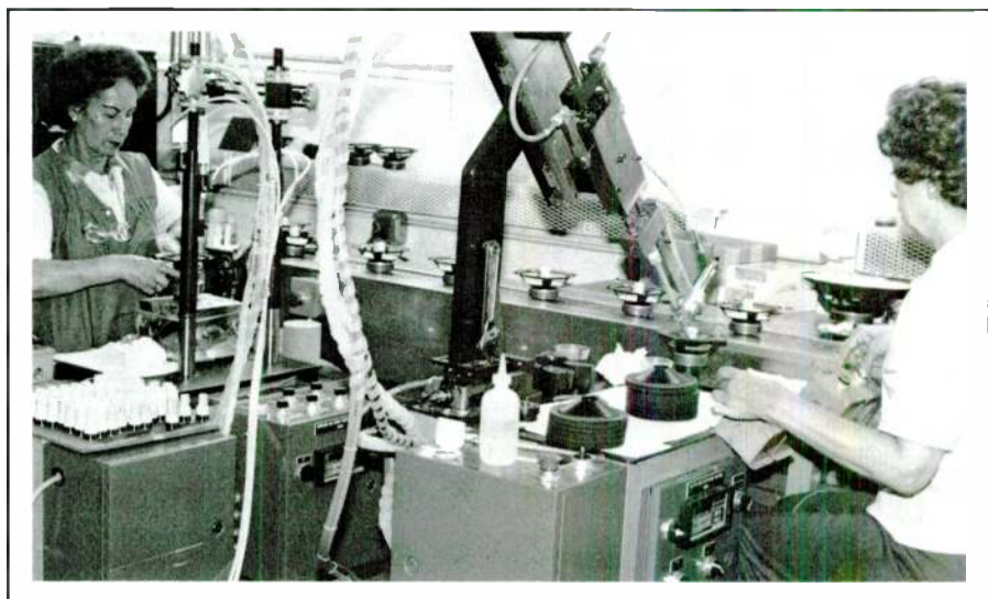
FIGURE 5: The operator on the left lays down two beads of adhesive on the basket for the outer edges of the spider and cone and inserts the spider and voice-coil alignment plug. The operator on the right lays in the cone and applies the adhesive for the spider-cone and voice coil interfaces in a two-step process.
