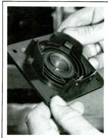
FIGURE 12: Andy Petite holds the voice coil/diaphragm assembly after it has been affixed in the tweeter frame.
