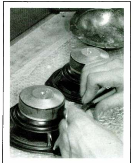
FIGURE 7: The alignment plug is removed, and flexible leads from the voice coil are attached to the input terminal strip.
