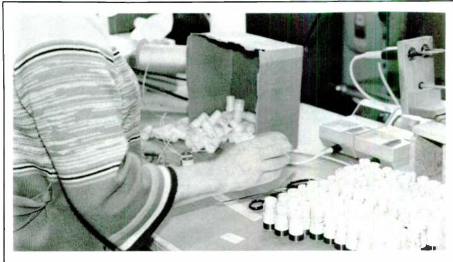
FIGURE 4: To assure alignment in production, the voice coil is inserted on a precision-formed plug.
