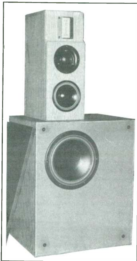
PHOTO 2: The subwoofer consists of a Dynaudio 30W54 12-inch woofer with a polysulfate cone in a 4.5-cubic-foot closed box. The height of the combined systems is 48 1/2 inches.
