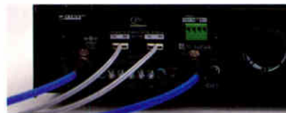
The plug-in QLink card is the EX amplifier interface, via fiber optic cable, to the Medialink network. It allows for several optional I/O modules, including MIDI, PA-242, RS-485, and other glass or plastic fiber optics.
