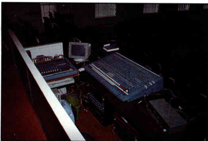
House mix position showing the Soundcraft Delta 200 main console along with the monitor console and the computer used for the IQ system.
