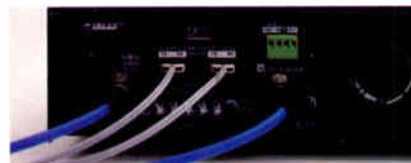
The plug-in QLink card is the EX amplifier interface, via fiber optic cable, to the MediaLink network. It allows for several optional I/O modules, including MIDI, PA-242, RS-485, and either glass or plastic fiber optics.
