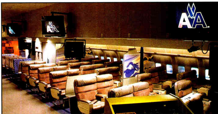
Aircraft simulator with overhead monitors and ceiling-mounted camera on sliding track, controlled by AMX Axxess system.
