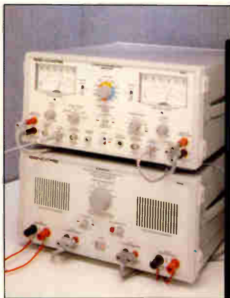
The PA81 can be used alone, or in conjunction with a scope and distortion analyzer.
