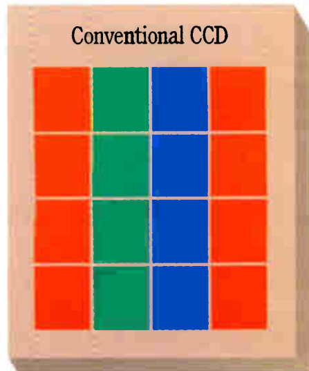
Conventional CCD: Red, green, blue "stripe" sensors can't resolve fine color detail, suffer from "channeling" when exposed to hot spots of light.
