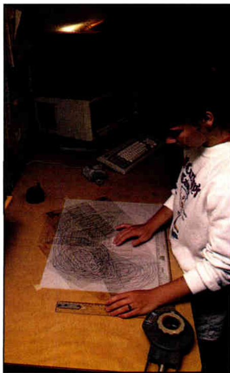
Isobars for various horns are selected and positioned for optimum coverage. Horn aiming angles are determined by the positions of the isobars on the map.
