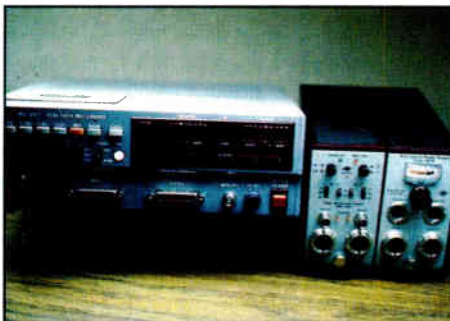
Tests were undertaken to determine the compatibility of the TEAC recorder and the B&K 1057 power supply.
