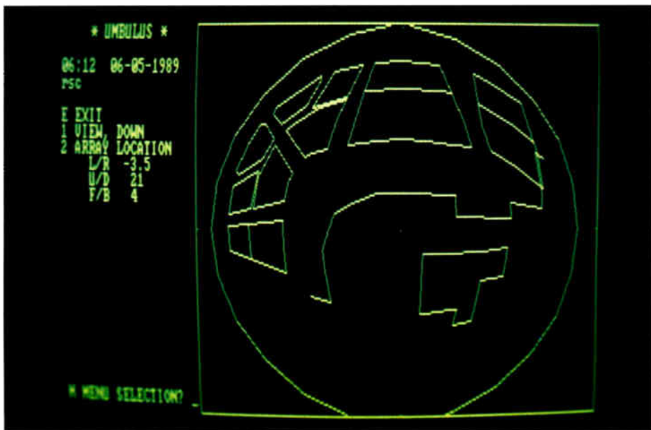
Here the room as seen from the array location. Umbulus offers users the ability to "fly" around the room, searching for a vantage point that gives an unobstructed view of all ear planes (as well as meeting other array location criteria).
