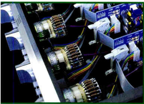
A look under the hood reveals the hand-soldered resistor networks.
