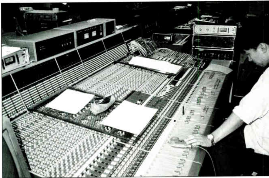
NHK's Concert Hall features a large control room equipped with a Neve VR Series and a customized Tamura console (pictured), designed in conjunction with NHK technical staff.
