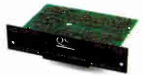
Optional accessory capability optimizes amps for bi-amplication of screen channels, protects surround speakers and equalizes the response of popular cinema subwoofers.
