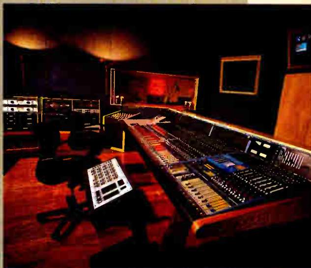
Mad Dog moved into a new, 3000-square-foot facility in Burbank, Calif. The Chris Pelanis-designed studio features a 48-in Neve 8108 with custom patchbay and Necam 96 automation, an MCI 2-inch 16-track and a Studer A800. Tielines connect to a 40x60-foot soundstage and a 1,000-square-foot recording room with three iso booths.
