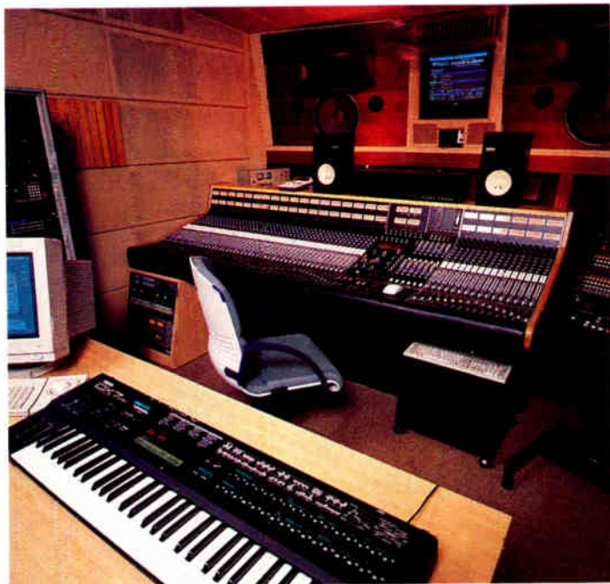
A 64-input API Legacy console with Flying Faders at Appo Sound, Tokyo
