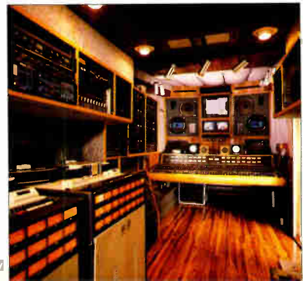
Record Plant Remote, West Milford, N.J.: Designed for 48-track analog or digital recording is the Record Plant Remote, of West Milford, N.J. Built into a 1990 35-foot Volvo FE-7 chassis, the truck features a custom Trident Series 80 48x32 console, UREI 813 monitors and an extensive synchronization system for handling broadcast, film or video dates.
