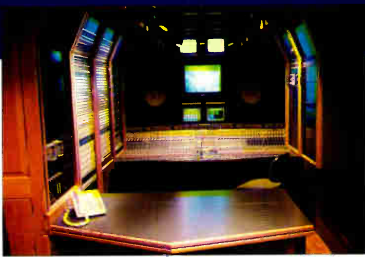
Remote Recording Services, Lahaska, Pa.: The Silver Truck has replaced the Black Truck at David Hewitt's Remote Recording Services, Lahaska, Pa. The 44-foot tractor-trailer includes an API 4848 console designed to Hewitt's specifications. KRK 15A-3 monitors cover the near-field. Design, of course, was by Hewitt.
