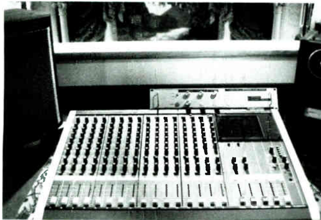
The Ramsa WR-S612 16-channel mixing console on the mezzanine level.
