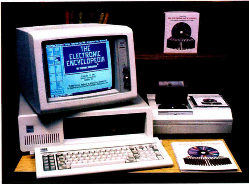
Personal computer (L) with software "engine" from KnowledgeSet; CD-ROM drive (R) with Grolier's Electronic Encyclopedia.
