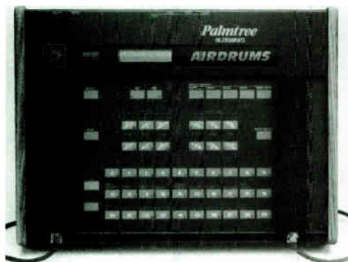
Airdrums from Palmtree Instruments (La Jolla, CA) is a new MIDI percussion controller consisting of a patch/note assignment editor-processor and two clave-sized, hand-held triggers with internal rotational accelerometers.
