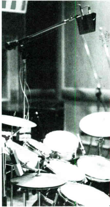
Drum miking arrangement for recent Ariel session at Tres Virgos: Back-to-back Crown PZMs in "wedge" configuration overhead; Shure SM-57 on snare; AKG 452s on toms; Sennheiser 421 on concert toms; Sennheiser 441 on high hat.
