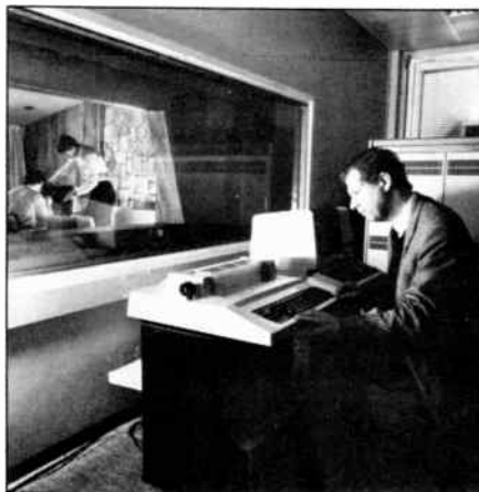
'Listening room' for the assessment of digital audio systems. A special wall separates the listening room proper from the control room for the computer used in digital-processing simulation.
