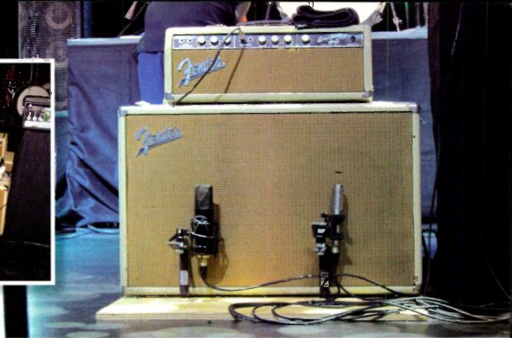
Brian Setzer Orchestra's engineer, Jimbo Neal (inset), places an R-121 a quarter-inch from the grille, roughly a half-inch off the dome, angled toward the paper cone about 30 degrees.
