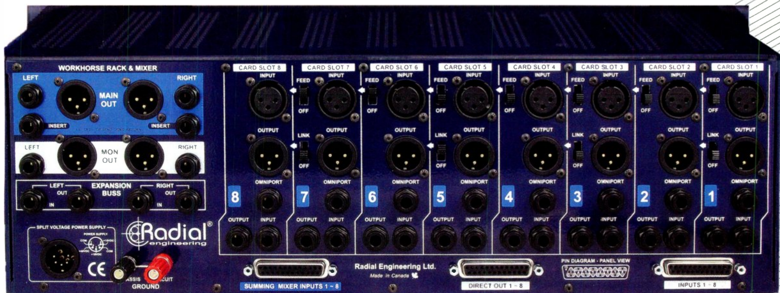
The Workhorse 500 also features an 8-channel mixer; back panel shown here.
