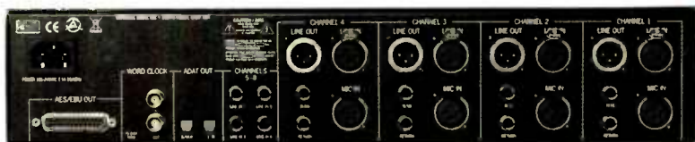
The back panel offers XLR mic in, line in and out, and balanced insert sent/returns on TRS plugs, as well as four extra TRS inputs for the extra line inputs.
