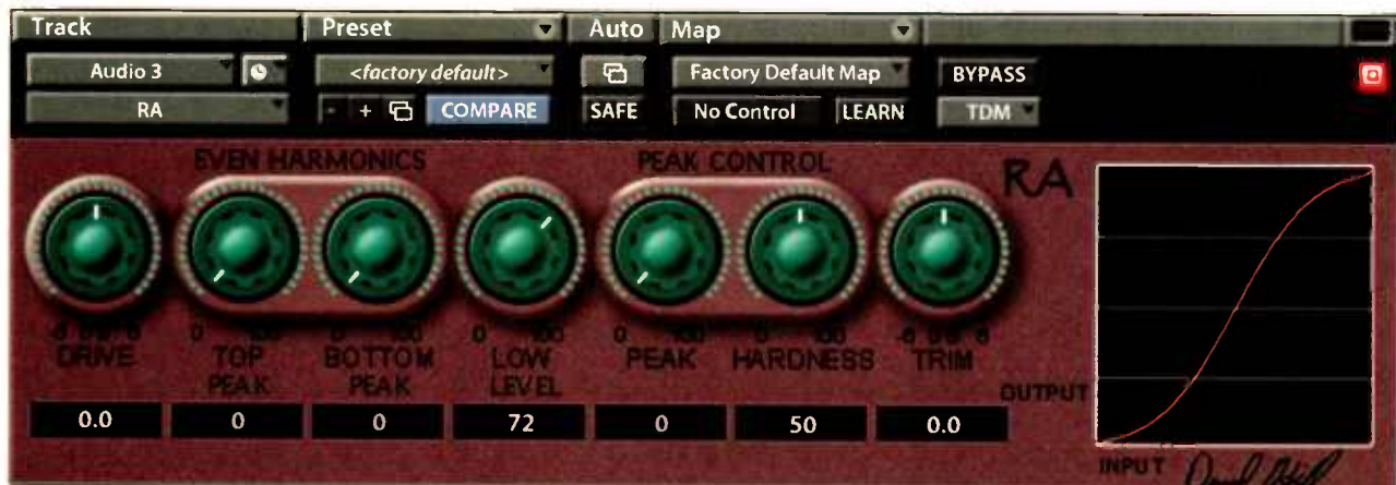
RA emulates amplifier overload, giving control over even harmonics, compression of low-level audio and peak level.
