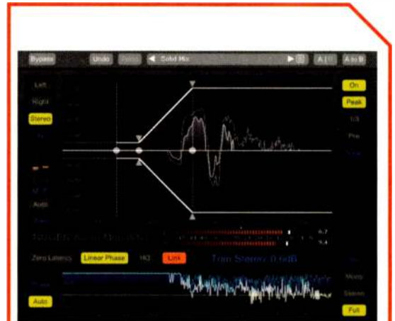
The Monofilter tightens low frequencies by forcing them to mono below the crossover point.
