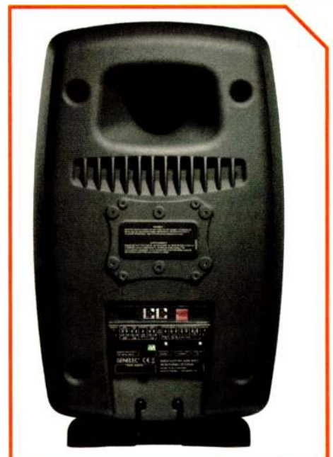
Rear panel controls include Bass Roll-Off, Bass Tilt, Desktop and Treble Tilt, and Stored or Manual controls.
