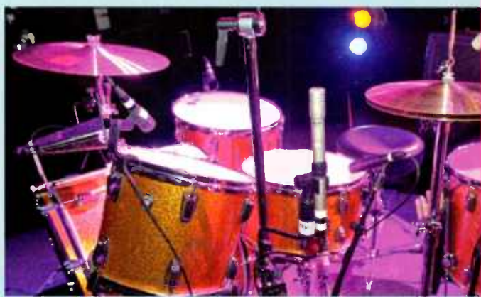
Patrick Carney's drum kit takes Shure Beta 91 and Beta 52 on kick; SM57 and Beta 56 on snare bottom and top, respectively; Shure KSM 137 (hi-hat); Sennheiser e 604s for rack and floor toms; SM81s on ride and crash cymbals, which are miked from underneath using LP claws; and an SM57 on cowbell.
