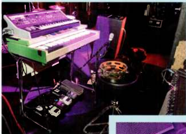
Backing on keyboards and percussion is Leon Michels. His keyboards include a Moog Little Phatty and a Farfisa, which are amped by a Fender Super Reverb miked with an SM57. Both keyboards go through Countryman DI boxes. A Beta 57 is on hand for tambourine.
