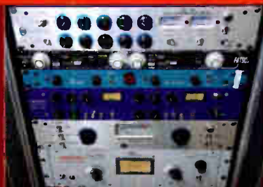
Analog treats (top-bottom): Summit Audio DCL-200 Dual compressor/limiter, Empirica! Labs EL-7 Fatso Jr., Ridge Farm Boiler ultra compressor. ("Serial number 35," says Carranza. "When you want something to go crazy, put it through that box."), Tube-Tech Dual Compressor CL 2A, Lindcraft Denmark tube stereo compressor, TLA-100A Summit tube leveling amplifier, and a Teletronix LA2A original limiter. ("When used with an amplifier, it zooms in on sound and brings out all the little characteristics that are in there.")
