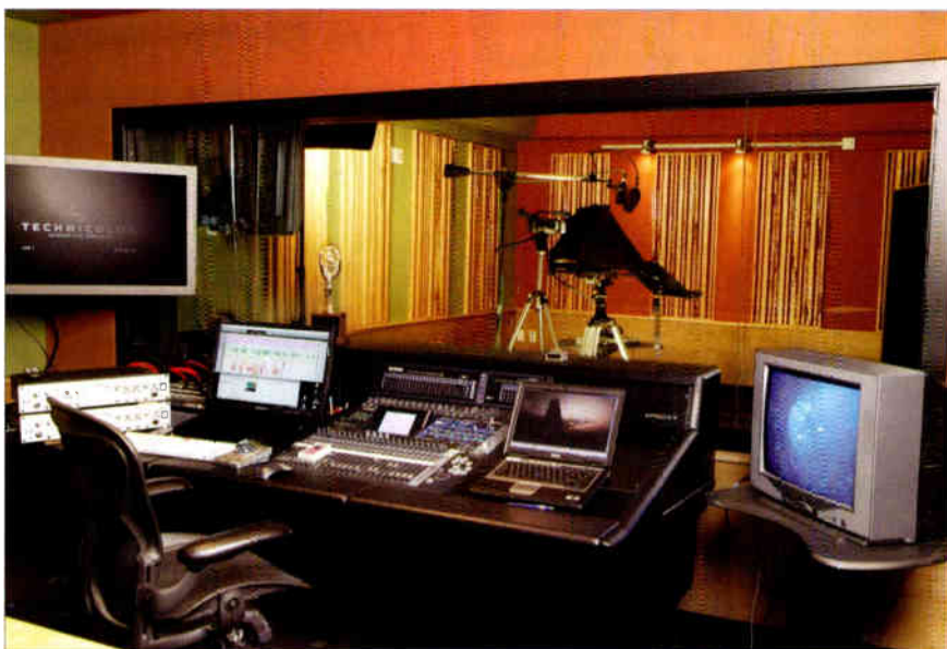
ADR 1, one of Technicolor's three voice recording stages, featuring a Yamaha O2R96 board, a pair of Avalon VT-7375P preamps and a custom teleprompter in the spacious booth. The three main edit rooms and mix room are all equipped with Pro Tools HD3.
