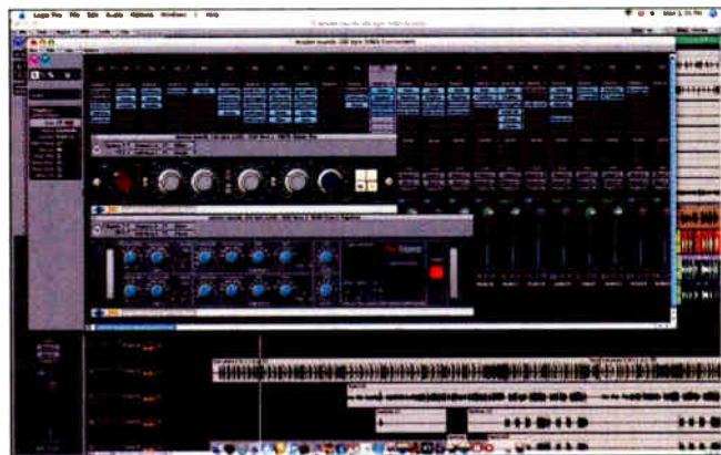
The UAD products let you effortlessly use massive, hardware-emulation plug-ins without taxing the host CPU. Here, the Neve 1081 EQ and 33609 limiter/compressor is running on a two-card system at 24-bit/48kHz with plenty of power to spare.
