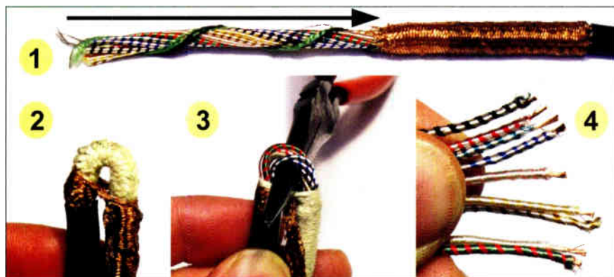
Figure 2b: How to prep a braided shield. Step 1: Compress the shield as far back as it will go. Step 2: Slowly bend the cable while poking through and stretching the shield until the underlying layer is exposed and a loop is created. Step 3: Poke through the loop with a rounded, blunt tool until the wires can be pulled through. Step 4: Separate and prep the wires for soldering.
