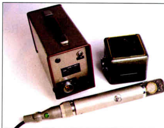
The modern C-414 hails from the original C-12, shown; the C-12A that followed it used a Nuvistor tube and debuted the familiar boxy body shape associated with the later 414 Series.
