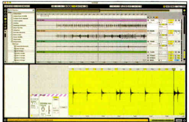
Live 6 lets users apply Warp markers across multitrack recordings at the same time. This feature is ideal for editing drums or imposing a single groove over multiple tracks of the same length.
