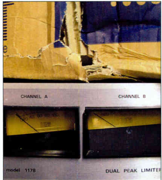
Figure 1: A UREI 1178 arrived in this box with a hole in it. The force was enough to dislodge the meters.
