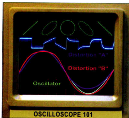
Figure 2: an oscilloscope display with a composite image of various waveforms (a simulation that is not possible in the real world). In green at top, the Lissajous patterns are the result of X-Y phase measurements. In blue, a square wave (far-left) as manipulated by equalization (or bad capacitors) to the right. At bottom, a sine wave (green) and two versions of distortion (violet and red).
