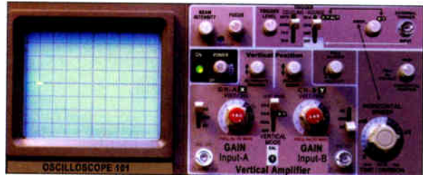
Figure 1: a simple dual-trace oscilloscope with a blank screen
