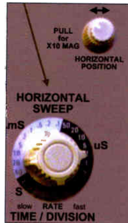
Figure 4: the horizontal sweep section of a 'scope
