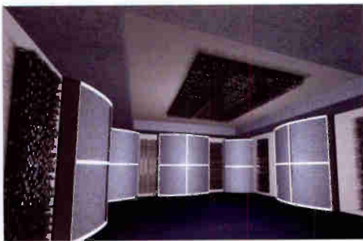
A rendering of the patented Chris Pelonis/RPG modular acoustical treatment system.
