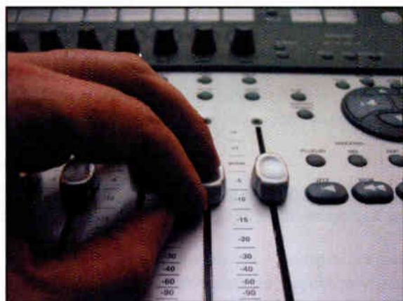
Fighting back with your middle finger: Try to nudge the 002's fader up, and it'll fight you because the front edge of its pad isn't touch-sensitive—that is, unless you rest another finger on top.
