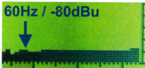
Figure 2b: Spectral analysis of the EMT-156 after power supply upgrade and modification.
