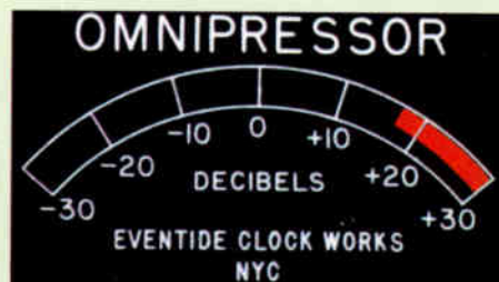
Figure 3: The Eventide Omnipressor can radically expand and compress. Note the 30dB swing (in each direction) on its zero-center meter face.
