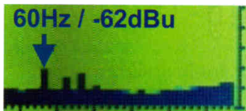
Figure 2a: Spectral analysis of the EMT-156 noise floor in "as-is" condition.
